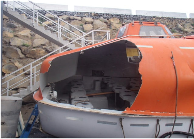
Figure 12: Lifeboat No. 5 Stern Damage
