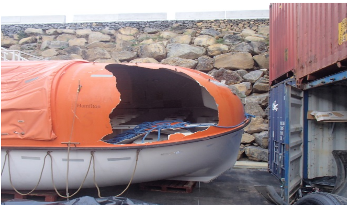
Figure 11: Lifeboat No. 5 Starboard Side Bow Damage
