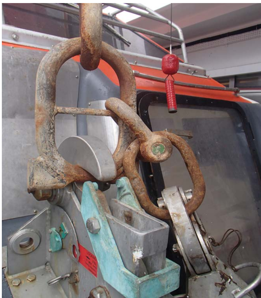
Figure 9: Image of a Tender Hook Arrangement. Note the lifting link centre stud and squaring at its base
