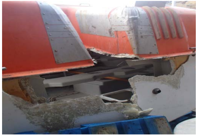
Figure 13: Lifeboat No. 5 Stern Damage – Note absence of aft hook
