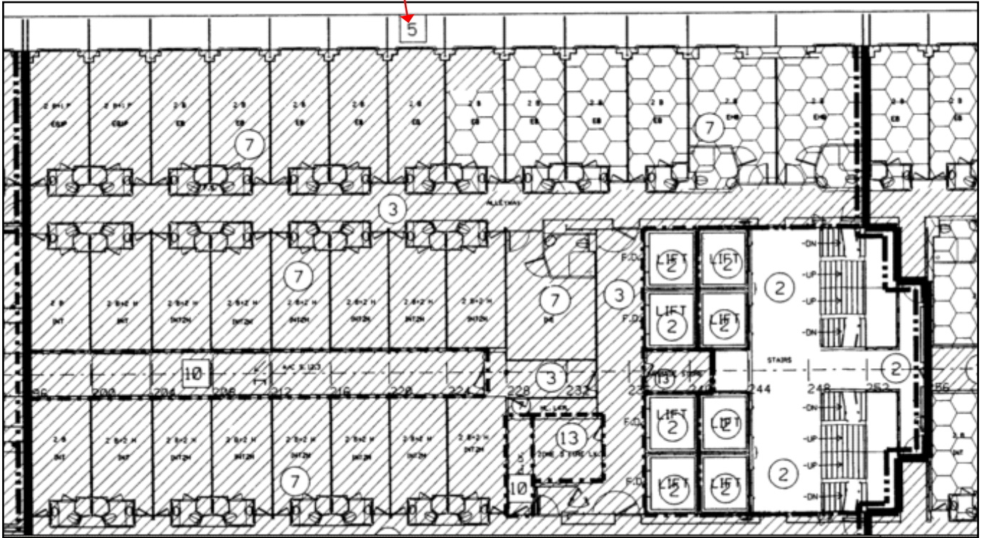
Extract of fire protection plan for deck 11 on Artemis (ex Royal Princess )
