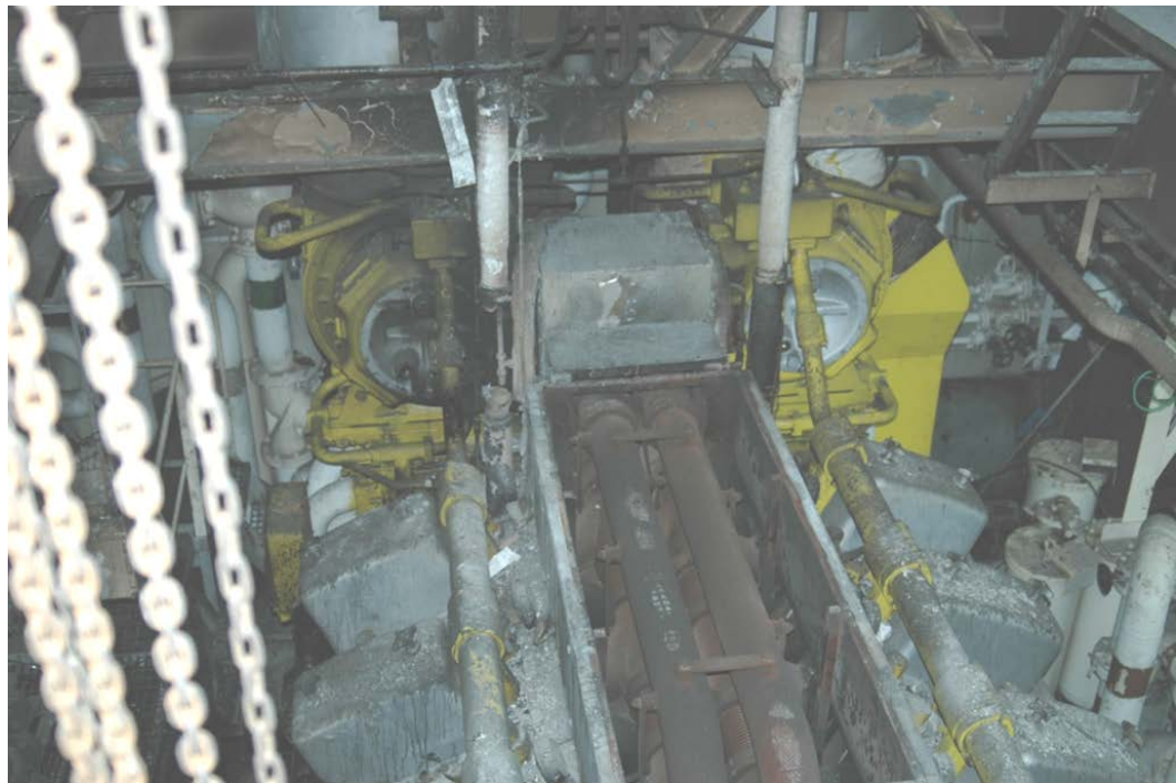
Engine No. 4 looking aft with the exhaust header covers removed. The seat of the initial fire can be seen in the scorching evident on the inboard side of the engine at the turbo charger close to where the cross over fuel lines enter the inboard hot box with evidence of scorching on the beam above.
