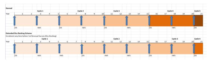
Once accepted onto the programme ships will be inspected in dry dock at intervals not exceeding  $7^{1}/_{2}$  years provided that two consecutive in-water inspections have been carried out. No extensions will be granted for the dry-docking required at the end of each extended dry-docking period.
